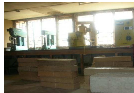
Figure 4. Hardened Beams stacked by numbers of reinforcements
