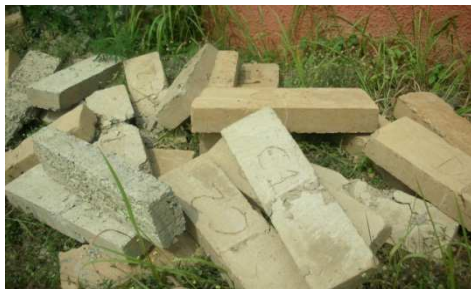
Figure 6. Failed Beam Specimens
