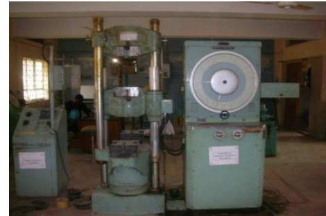
Figure 3. Avery Denison Universal Testing Machine
